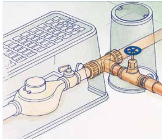
P.O.C. Non-Freezing: Use a brass compression tee to connect your sprinkler system to the household water supply.
