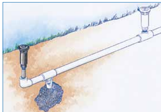
Automatic Drain Valve Installation for Freezing Climates: Locate the drain valves at the low points in each zone.
