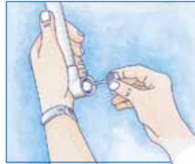
Assembling PVC: 1. Place solvent on inside of fitting and outside of pipe.
