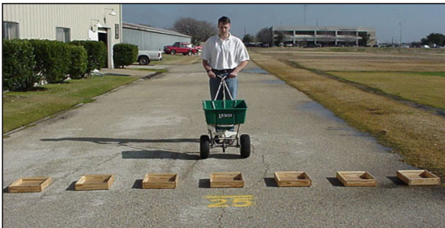
Figure 6: Set out catch pans to equal distances from the center point to catch fertilizer at the edge of the throw pattern. Image from Texas A&M University
