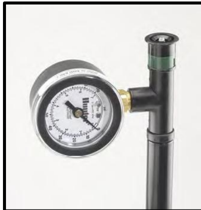
Dynamic pressure w/ gauge for spray bodies
