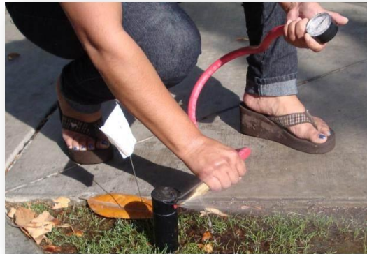
Dynamic pressure w/ hose and pitot tube
