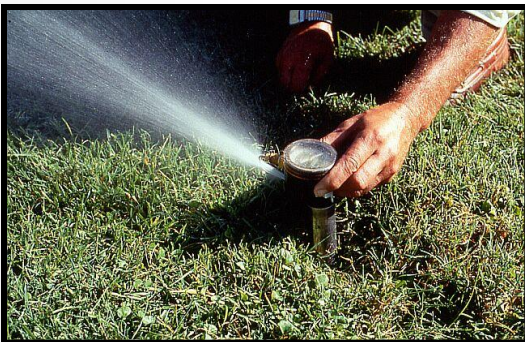
Dynamic pressure w/ pitot tube
